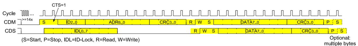
Figure 13: Register write access
