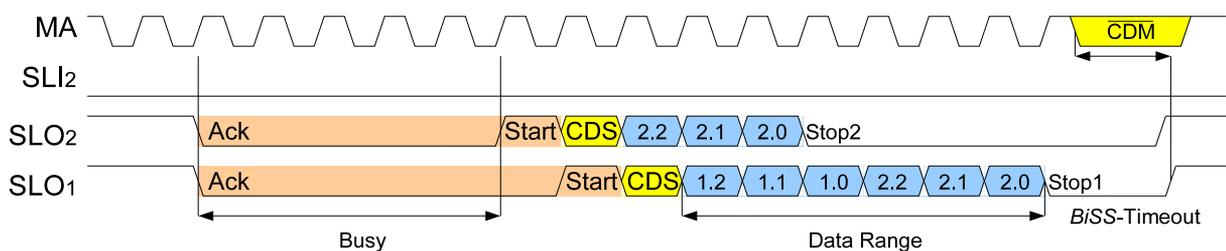
Figure 3: Requests for processing time (point-to-point configuration)
