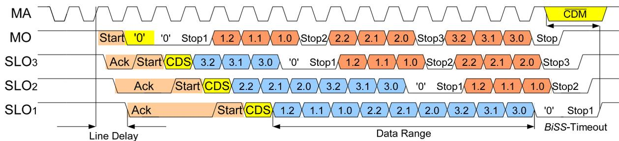
Figure 5: Line delay compensation by the master
