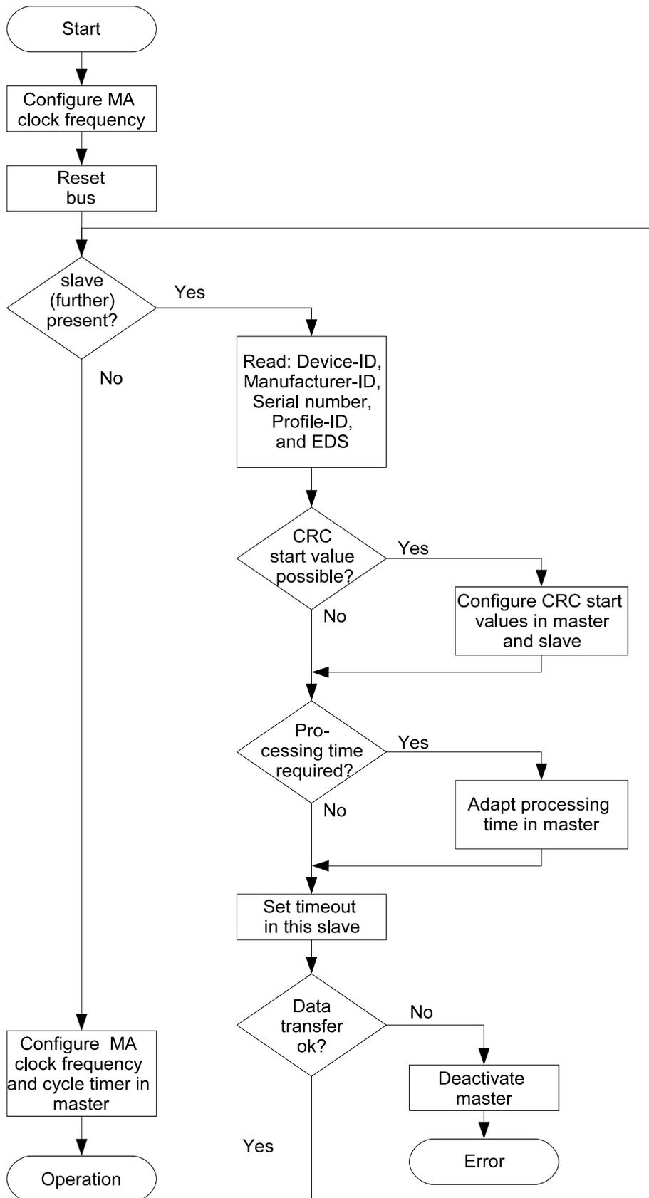
Figure 20: Procedure for a bus establishment
