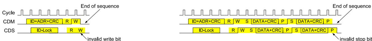
Figure 17: Accesses to non-implemented registers (here Write)
