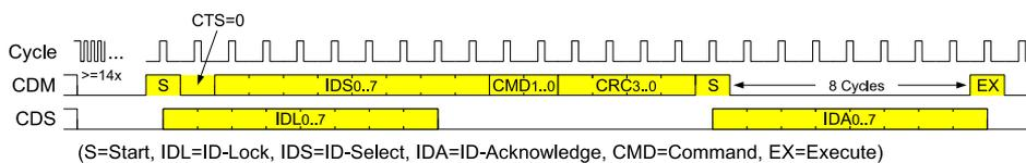
Figure 11: The command frame (addressed)
