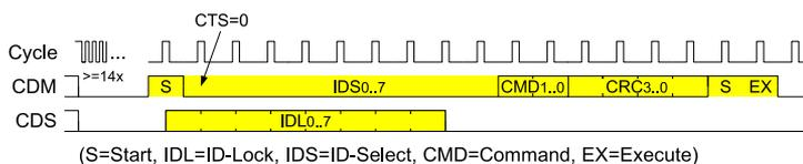
Figure 12: Command frame (broadcast)
