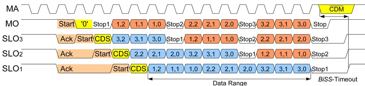
Figure 2: *BiSS* frame with 3 slaves (bus configuration)
