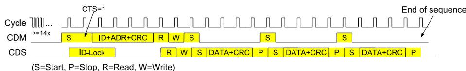
Figure 16: Reading several register
